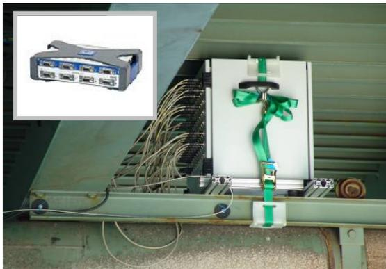
**Fig. 6:** QuantumX amplifier system (HBM) installed in a robust box in measurement section 5 below the bridge
