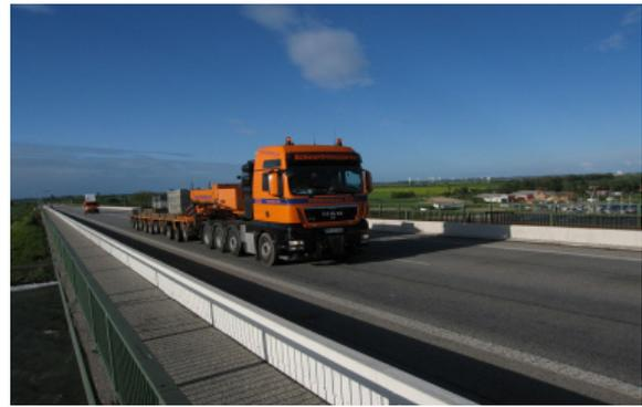
**Fig. 7:** Heavy-duty truck with additional 120 t load
