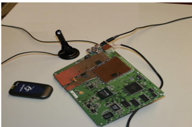
Figure 5: The used standard modem to measure SCORE values. The Omni-directional antenna and the GPS receiver are also shown
