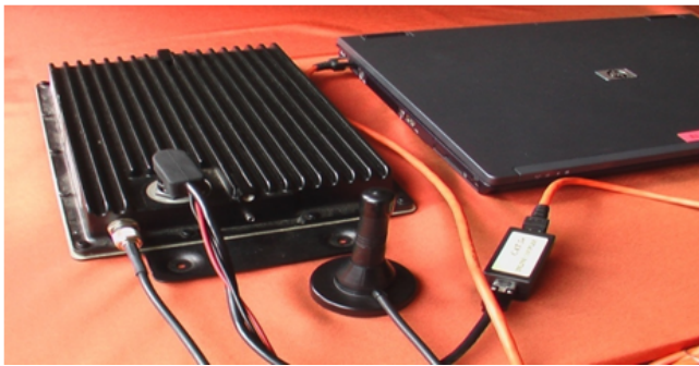
Figure 4: The used modem to measure RSSI, with the used Omni-directional antenna
