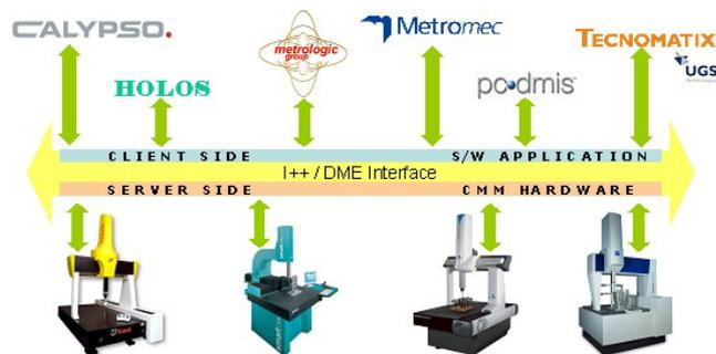
**Fig. 4: Interoperability test of the I++ DME interface**
