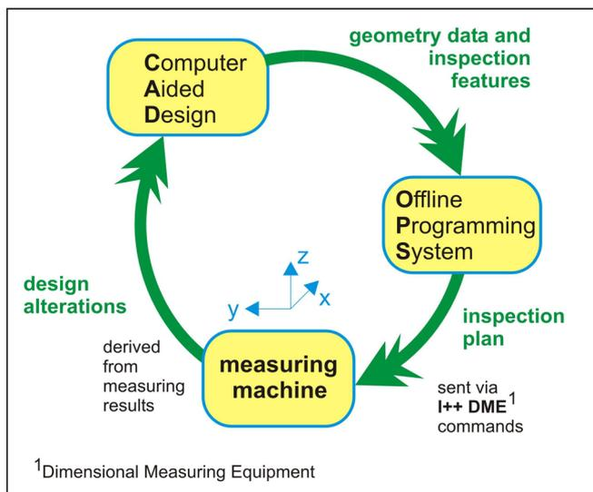
Fig. 2: General setup of a closed quality loop for dimensional measurements with coordinate measuring machines (CMM)
