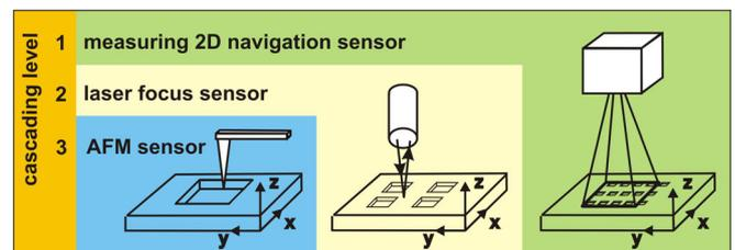
**Fig. 5: Setup of a cascaded multisensor system**
