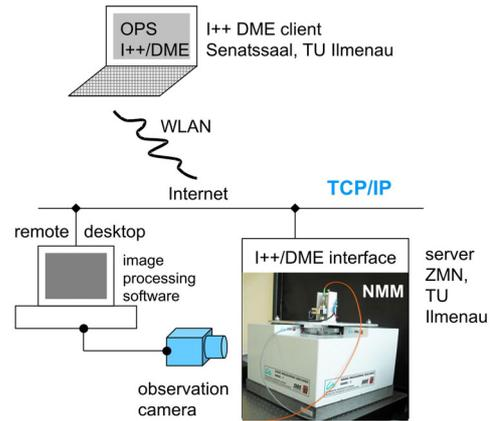
Fig. 6: Experimental setup for the demonstration of the remote execution of an inspection plan via the I++/DME interface [21]
