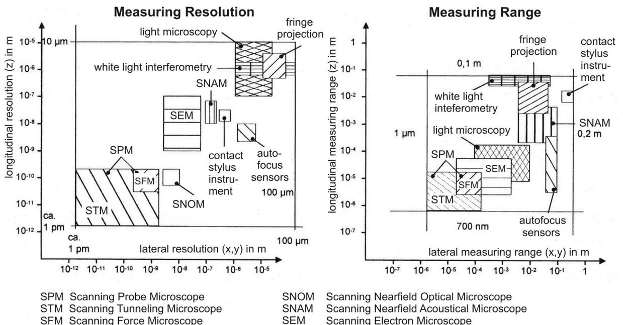
Fig. 1: Resolution and measuring range of typical measuring methods for micro- and nanoscale components [15]
