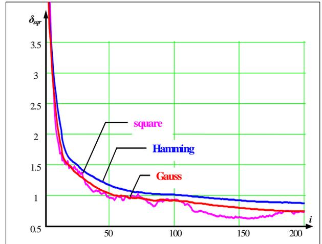
**Fig.6. Relative mean square filtration error for: square, Hamming and Gauss windows**
