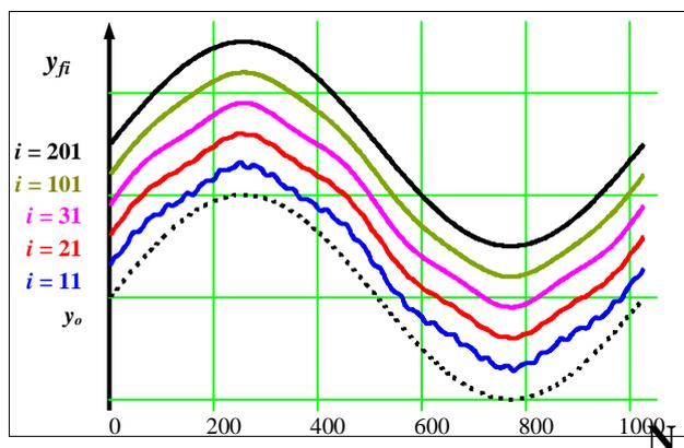
**Fig.10. Weight filtration of the random noise with Hamming window (for different windows width)**
