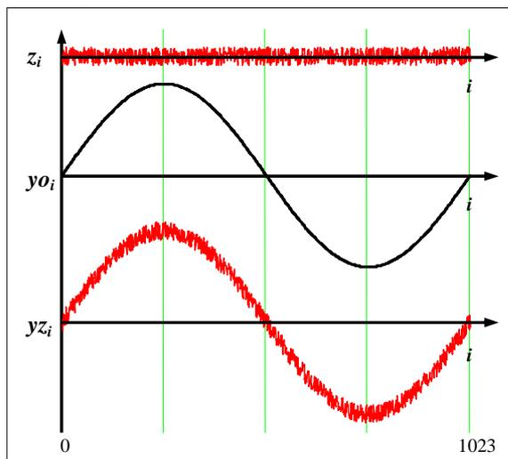
**Fig.2. The input signal  $y_o$  disturbed by a random noise**
