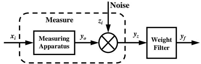
**Fig.1. The model of the measure procedure**
