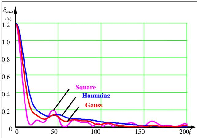
**Fig.8. Relative maximal filtration error (square, Hamming and Gauss windows) for periodical disturbances**
