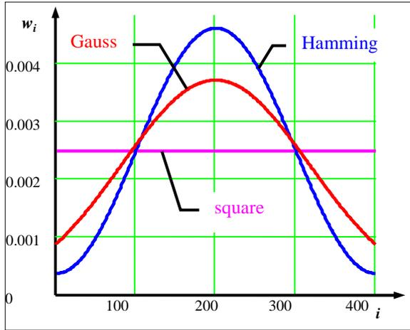
**Fig.4. Samples of weight windows: square, Hamming and Gauss**
