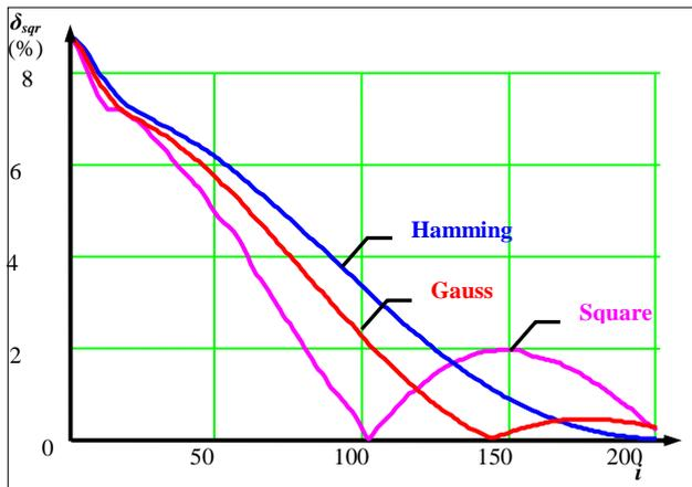
**Fig.9. Relative mean square filtration error for: square, Hamming and Gauss windows**
