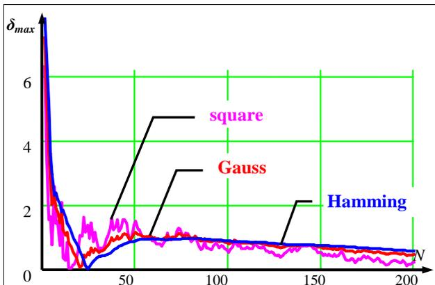
**Fig.5. Relative maximal filtration error (square, Hamming and Gauss windows) for random noise**
