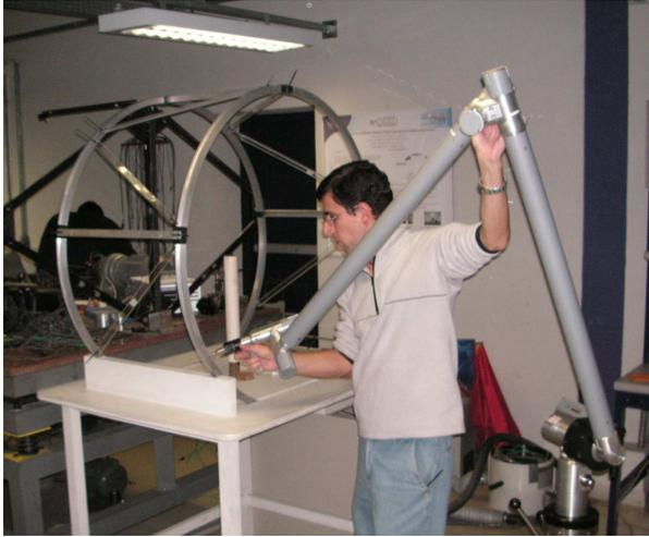
Figure 5 – Coil dimensional measurement using the CMM arm.
