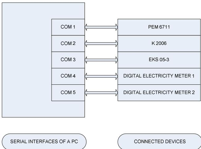
Fig. 3. Connection of the devices to the master PC.
