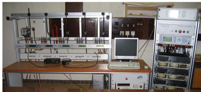
**Fig. 2. Photograph of the calibration laboratory with electronic calibration station EKS 05-3.**
