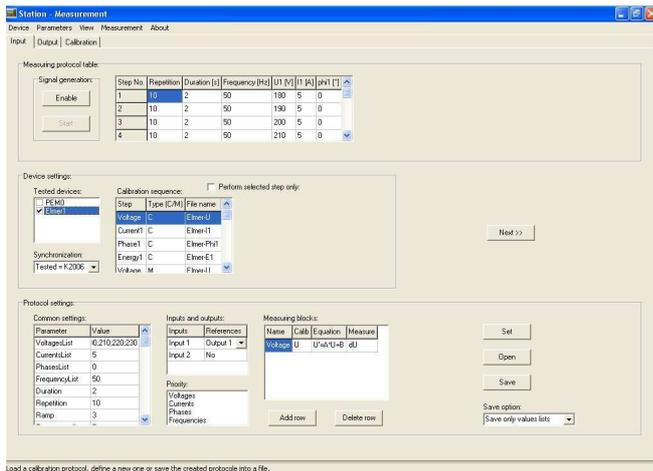
Fig. 5. Screen shot of the program Station – input settings.
