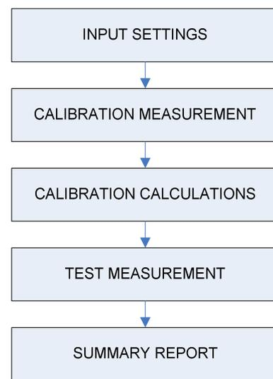
Fig. 4. Steps of the automated calibration process.
