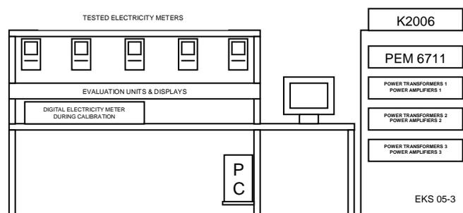
**Fig. 1. Schematic drawing of the calibration laboratory with electronic calibration station EKS 05-3.**
