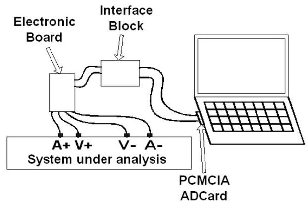
Fig. 4. Block diagram for the measurement setup.
