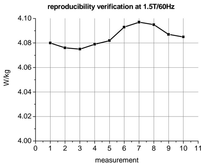
Figure 2. Losses at 1.5T/60Hz for reproducibility verification
