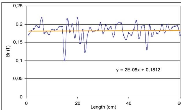
Fig. 6. Remanence magnetization  $B_r$  versus fiber length
