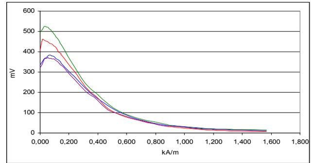
Fig. 7. The first derivative of the  $\lambda$ -H response at various points of a stress current annealed ribbon
