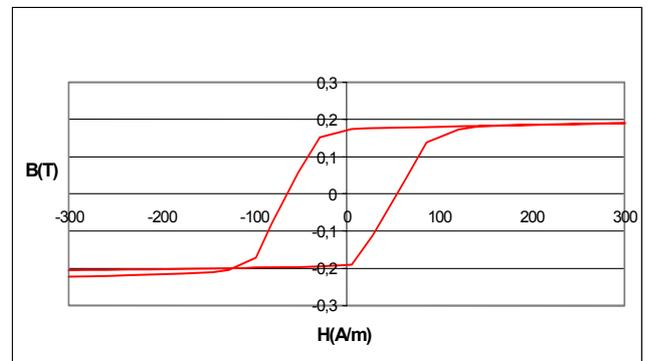
Fig. 3. Typical B-H loop for a stress-current annealed amorphous fiber
