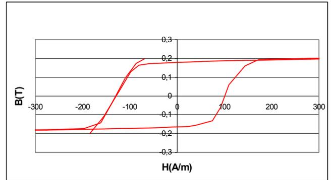
Fig. 2. Typical B-H loop for an as-cast tested amorphous ribbon
