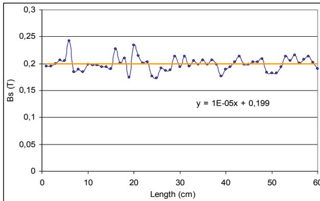
Fig. 5. Saturation magnetization  $B_s$  versus fiber length
