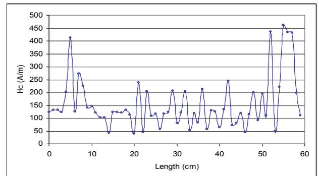
Fig. 4. Coercive field  $H_c$  versus ribbon length
