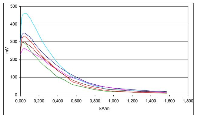
Fig. 8. The first derivative of the  $\lambda$ -H response at various points of a stress current annealed wire
