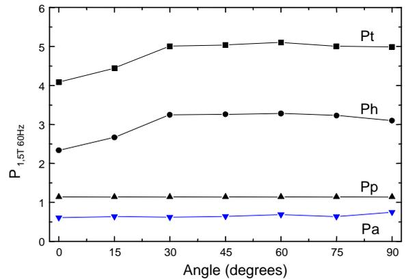
Figure 5. Losses - total, hysteresis, eddy and anomalous as function of the angle to RD.  $B=1.5T$ ,  $f=60Hz$ . Epstein.
