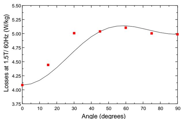
Figure 2 Experimental results for iron losses at 1.5 T / 60Hz (points) compared with equation (4) (full line).
