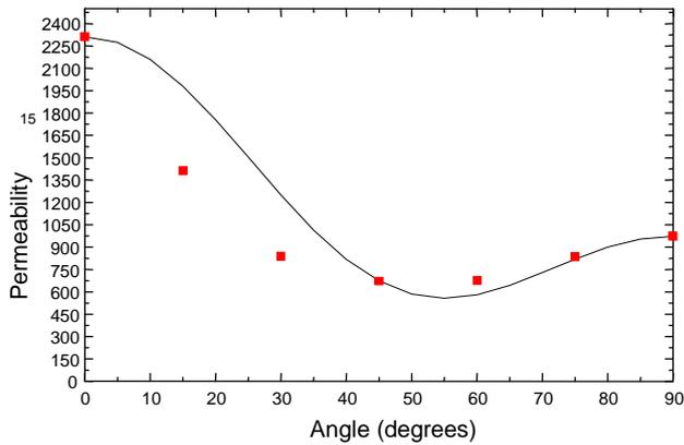
Figure 3 Experimental results for permeability  $\mu_{15}$  (points) compared with equation (5) (full line).
