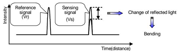
(b) Reflected signals from reference mirror and sensing mirror
