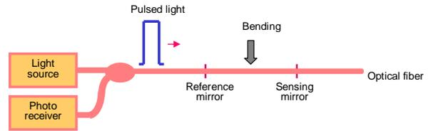
(a) Schematics of optical loss based fiber optic sensor
