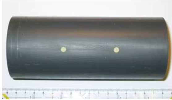
Fig. 3. Test plug for fall experiments with perturbation
