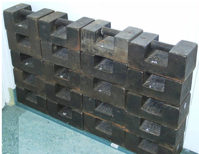
Fig. 2. Set of weights (20 kg) for calibration of weighing instruments
