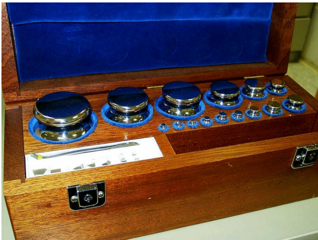
Fig. 3. A set of weights (1mg-2 kg)
