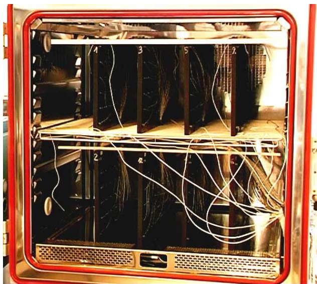
Fig. 2. Calibration in temperature chamber
