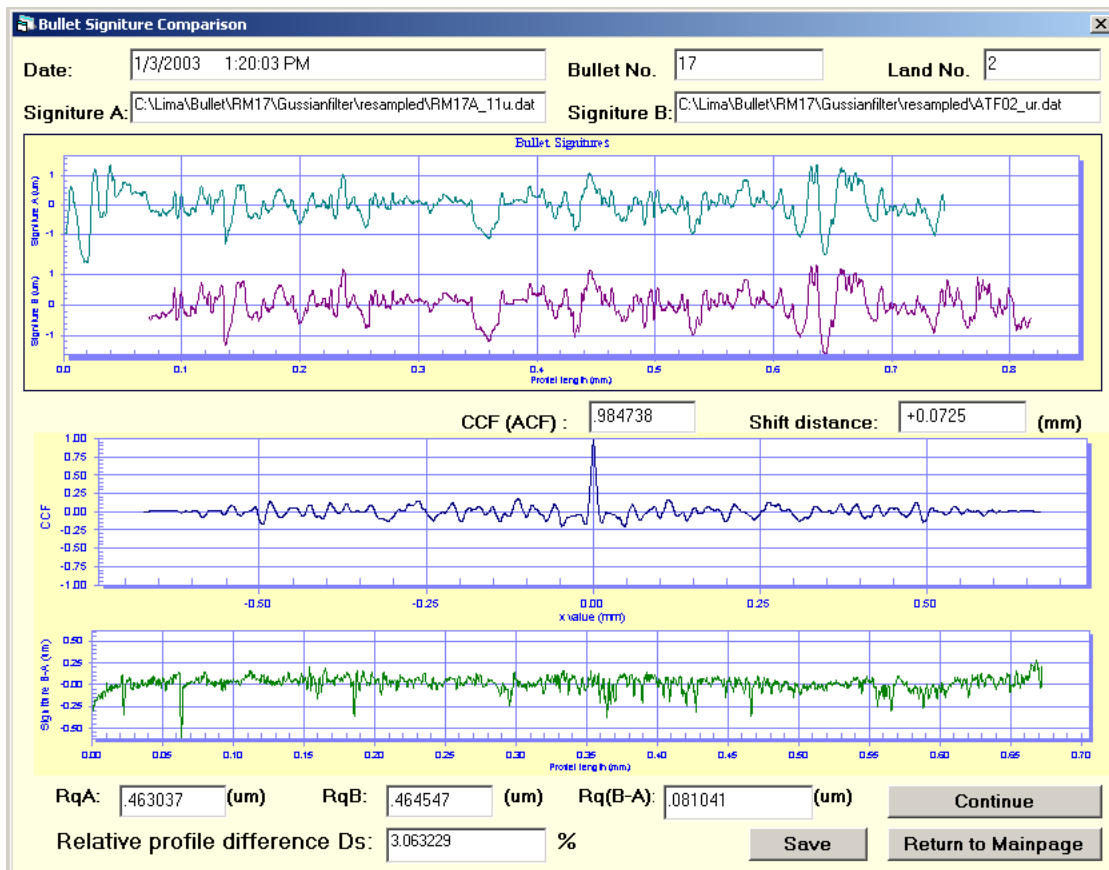
Fig. 2 Two compared signatures A and B with the same signature pattern but shifted in the lateral direction. There is a correlation peak on the CCF curve. Signature B – A shows the difference between Signature A and B.
