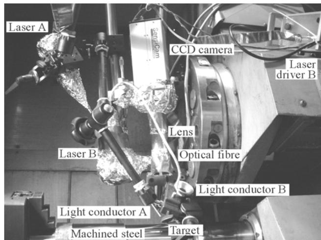
Fig. 2. Measurement system. Two laser heads and CCD camera were attached to the moving tool chunk.
