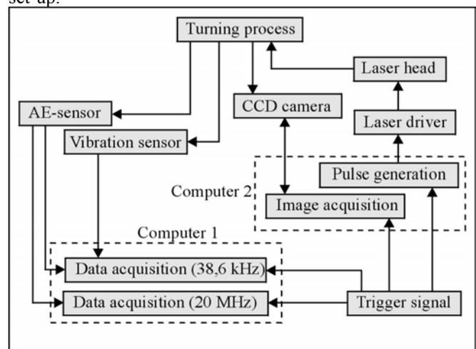
Fig. 1. Experimental set-up for diagnosis of the turning process. PC 1 was used for acquisition signals from AE and vibration sensors and PC 2 was operating the laser illumination unit and simultaneous image acquisition via CCD camera.
