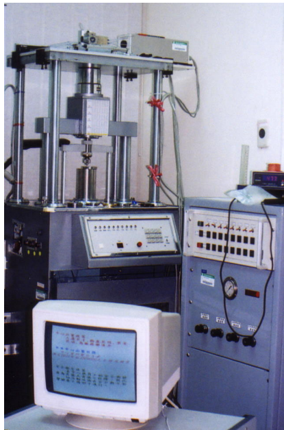
Fig. 2. Primary Rockwell Hardness Standard System in CMS.
