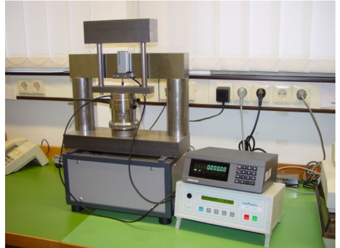
Fig. 7 Calibration of the depth calibration device with the help of the line scale reference device
