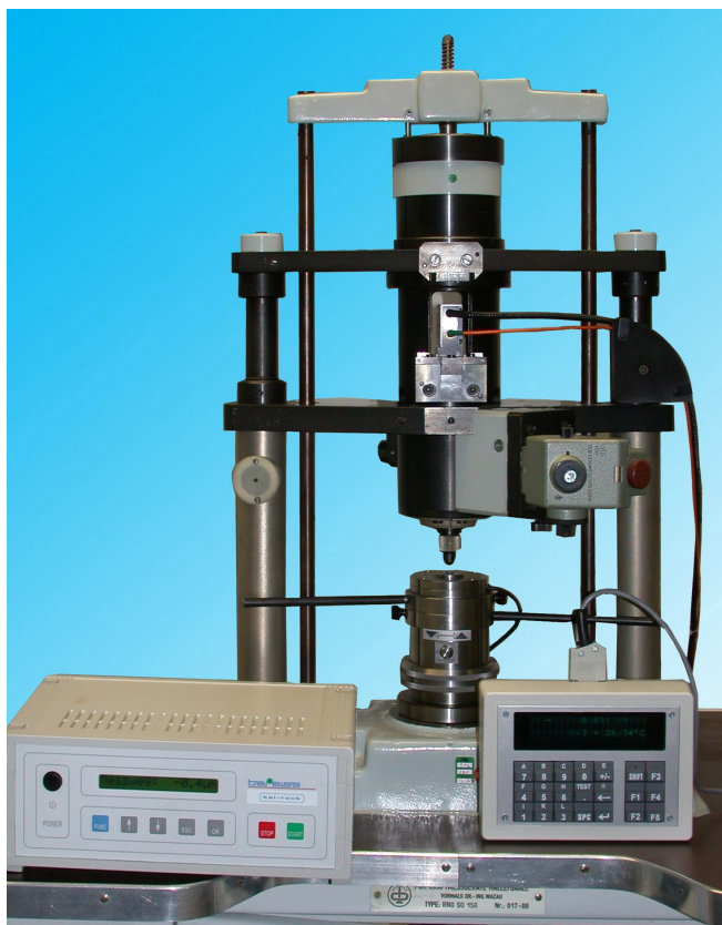
Fig. 2 Calibration of the depth calibration device with the help of the Rockwell hardness standard machine
