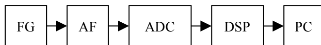
Fig. 3. Block diagram of research set; FG – function generator (Agilent 33120A); AF – antialiasing filter; ADC – analog to digital converter ( \Sigma\Delta 16 bits); DSP – digital signal processor (ADSP-21061 of Analog Devices); PC – PC computer
