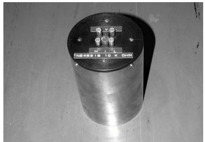
Fig. 3. Four terminal-pair ac resistance standards compared.
