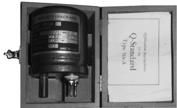
Fig. 4. Tested Q-standard, type 518 A
