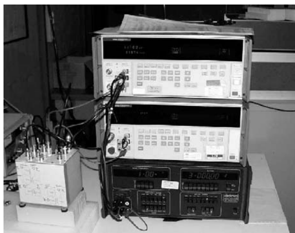
Fig. 7 Calibration of a precision ac voltmeter in the millivolt range in comparison with another ac voltmeter and the wideband transformer.
