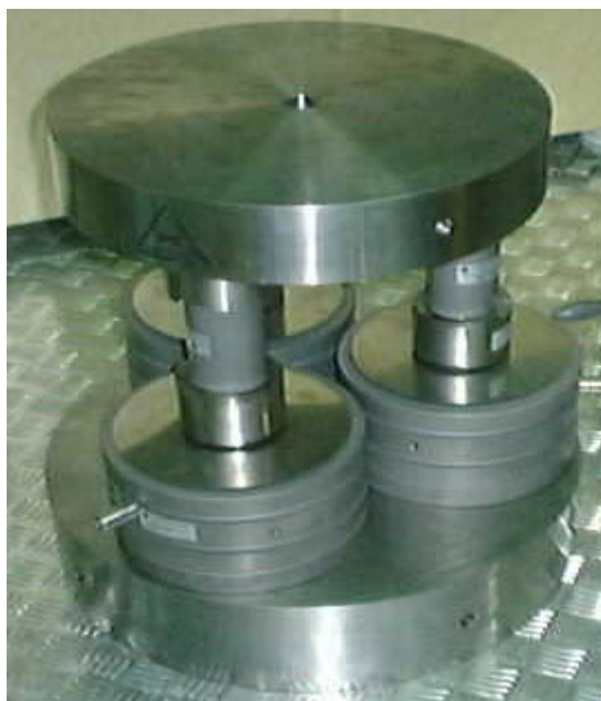
Fig. 3. 3 MN Build-up force transducer of UME
