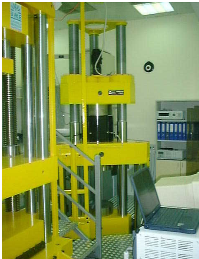
Figure 1. 3 MN hydraulic type build-up force standard machine of UME Force Measurement Laboratory
