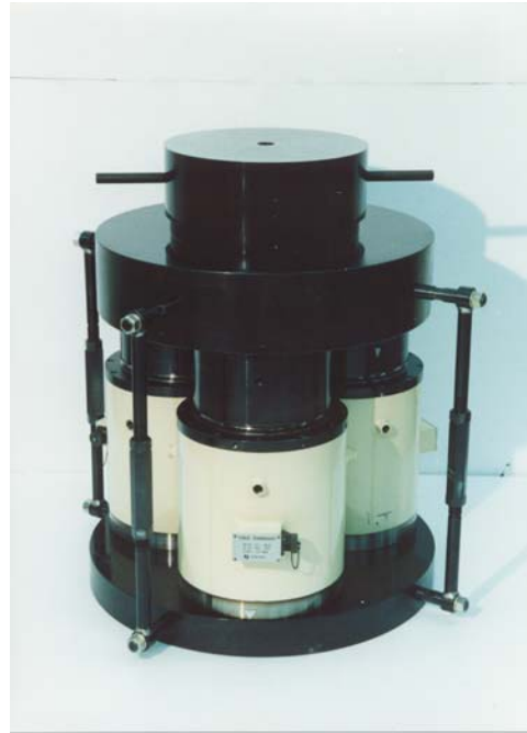
Fig. 3 Photograph of 30 MN build-up system
