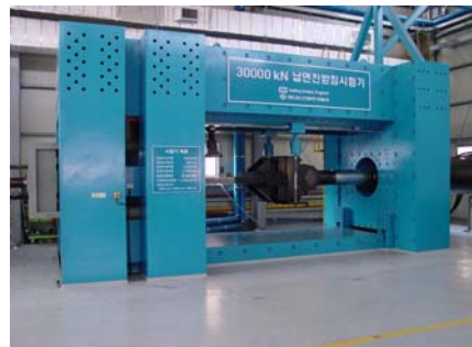
Fig. 4 30 MN pot bearing testing machine
