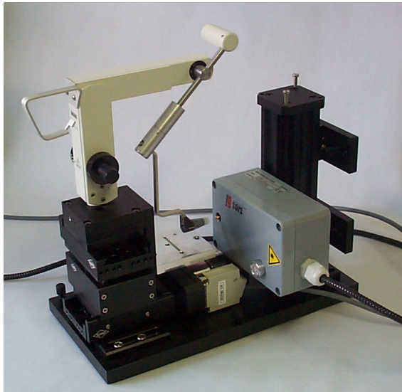
Fig. 2: Interference-optical check equipment for tonometers
