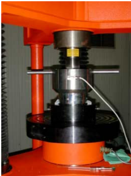
Fig. 4: Single load cell calibration on the IMGC-CNR 1 MN deadweight machine
