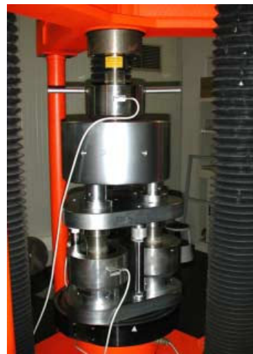
Fig. 5. IMGC-CNR - Force standard machine of 1 MN with the 3 MN Build-Up Force Transfer Standard
