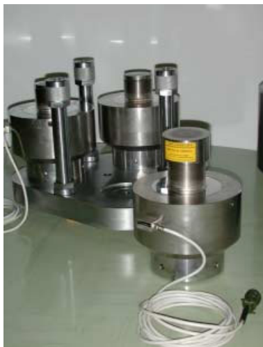
Fig. 1. The three force transducers analysed and calibrated for the Build-up prototype
