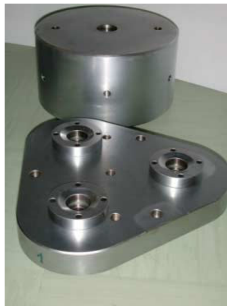
Fig. 3: Base plate and loading plate
