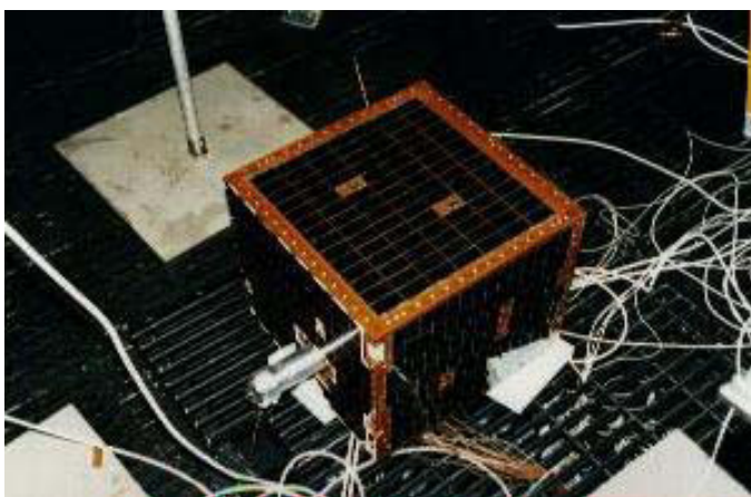
Fig. 2. SEDSAT-1 in the test chamber, with PALADS sticking out
