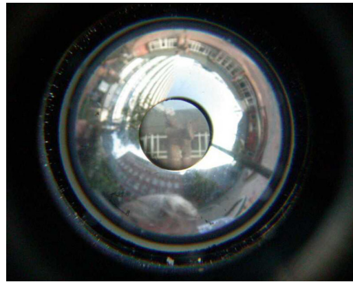
Fig.6. Foveated image shows a four times magnification of a selected part of the 360° panoramic image
