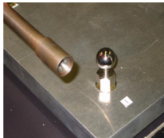
Fig.6 The cone-shaped stylus is approaching the ball
