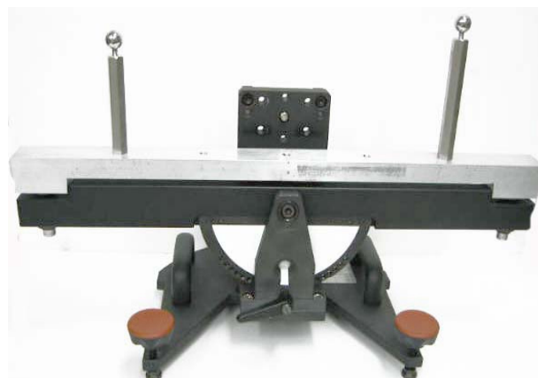
Fig.4 Simple artifact with two spheres. The distance between two spheres is about 400mm. The basement of the spheres can be tilted.
