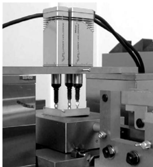
Fig. 8 Photograph of measuring method of tilt angles of X stage
