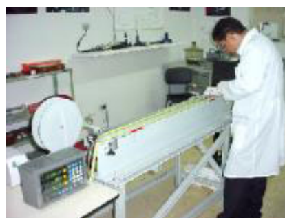
Fig. 6. Tape calibration using digital method
