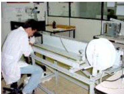
Fig 2. Tape Calibration using analogical method
