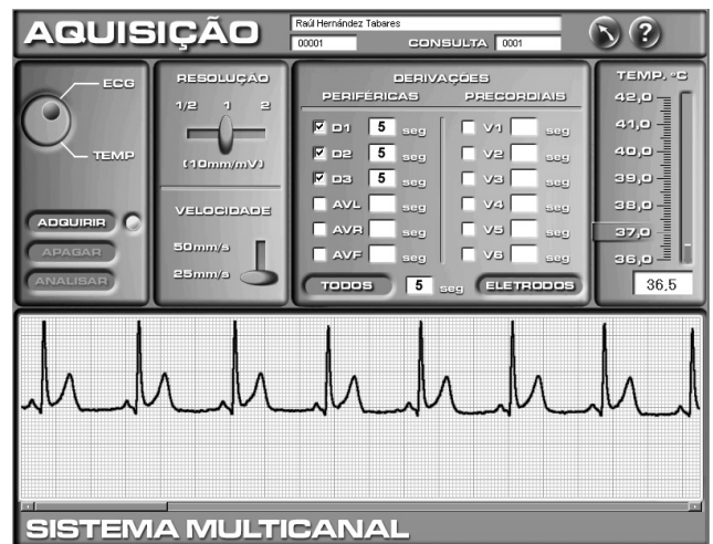
Fig. 4: Main window of the program for acquisition and storage of bioelectric signals for the SABIO electro-cardiogram system.
