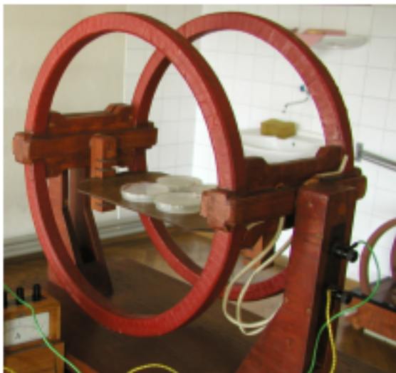
Fig. 4. Lemna minor inside Helmholtz coil
