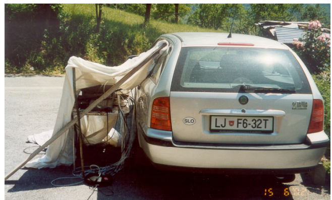
Fig. 5a (temperature), 5b (relative humidity), 5c (measurement set-up) in Škoda Octavia combi, metallic silver, closed windows, 100 % clear weather, with and without air-condition
