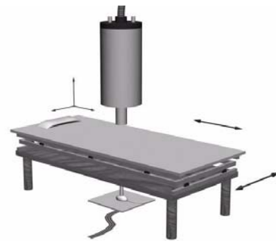
Fig. 1: Experimental set-up used for localisation of steel needles.
