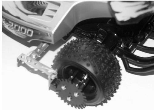
Fig. 3. Custom design for r.p.m. sensor.
