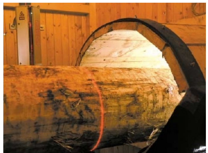
Fig.4: Projected laser beam on log for the 3D-method
