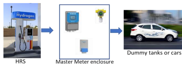
Figure 1: Master meter method for on-field verification of HRS
