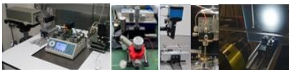
Figure 1. Micro flow calibration techniques. Left: interferometric method. Middle: volumetric method. Right: pendant drop and front track method.
