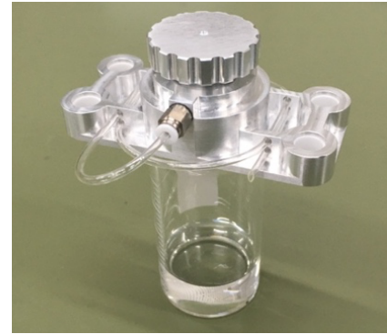
Figure 3: Photo of the weighing tank with the slender tube.
