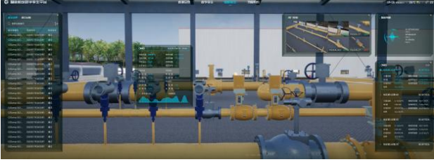
Figure 3: Actual diagram of auxiliary simulation verification of digital twin platform for intelligent verification of natural gas metering
