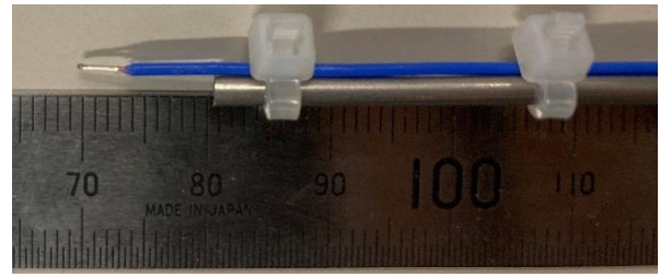
Figure 1: Thermocouple used in experiments (Wire diameter: approximately 300 μm).
