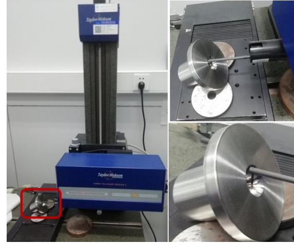
Figure 1: High-precision surface roughness instrument.
