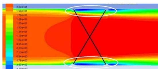
Diagram 4 Variation of Flow Field in Pipeline after Probe Goes Deep Into Pipeline and Forms Bulge
