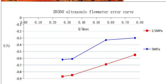
Diagram 1 Verification of ultrasound test results at 2.5 MPa and 5 MPa
