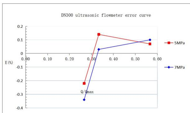
Diagram 2 Verification of ultrasound test results at 5 MPa and 7 MPa
