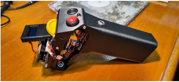
Fig. 1 The PICUS device without the outer protective covers in order to observe the composition of the system interior.
