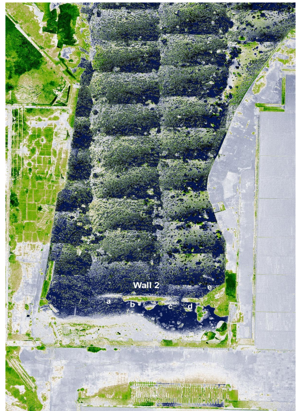
Fig. 8. NDVI Index Map from Multispectral Drone Survey: The Wall 2 identified through different growth of algae. |© G. Cacciaguerra and S. Barone - CNR ISPC.
