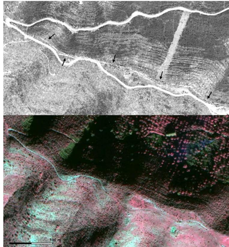
Figure 7. Phoenike. Sections of the ancient walls line clearly visible in a georeferenced KH-9 Hexagon space photos of 1975 (above); the same sections of the walls, little or not at all visible, in a false color RGB composition of pancharpened image obtained by datafusion of panchromatic and multispectral data of a GeoEye-1 (below).
