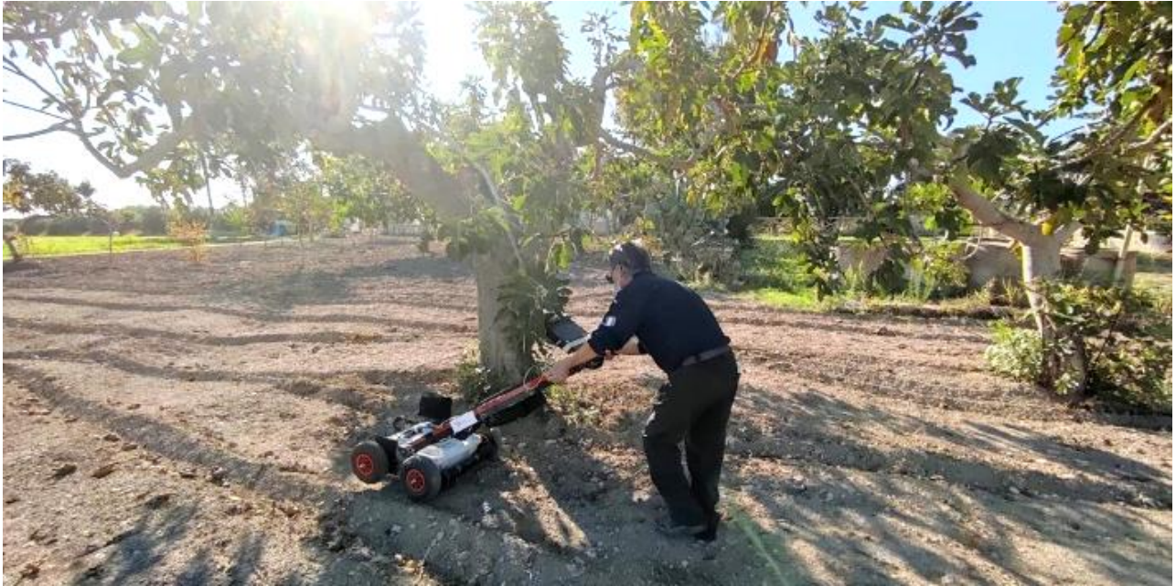
Fig. 3. Photo relating to the measurement phases with a GPR.
