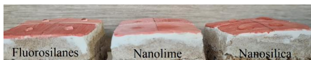
Fig. 2. Example of wettability of formulations applied on mock-up samples prepared with the fresco techniques.
