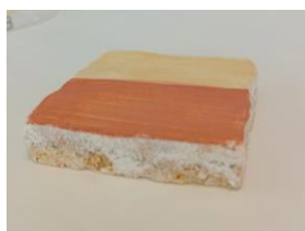
Fig. 1. Example of mock-up painted samples simulating the fresco.
