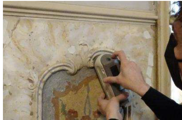
Fig. 3. Execution of a spectrophotometric analysis on the right panel of the boiserie.
